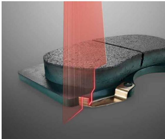
The relative position (height) of the tip of a brake pad wear indicator and the brake pad surface is measured.
