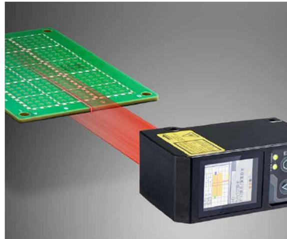
As opposed to a displacement sensor in which thickness measurements are performed using two substrates on top of one another, LS series sensors can measure one substrate from the lateral direction, enabling feasibility in terms of both mounting and designing.
