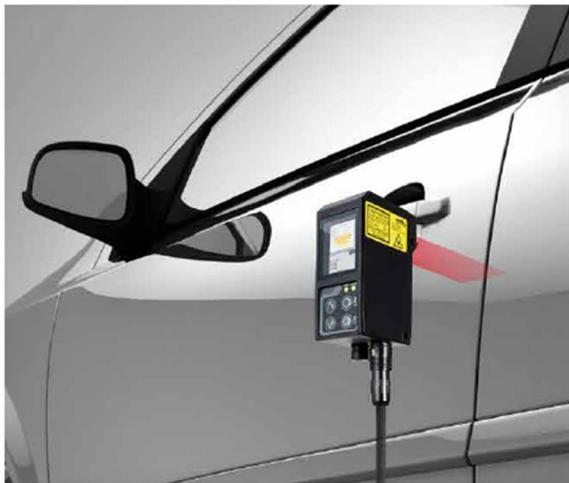
In order to confirm accuracy when installing doors on vehicles, non-contact measurements are performed quickly using the gaps and height differences between the doors and vehicle body.
