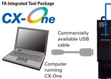
The built-in USB port lets you connect to a personal computer using a general-purpose cable.
