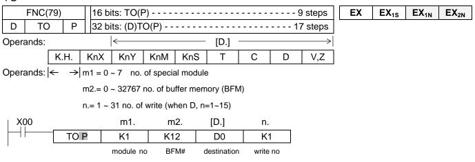
♦ When X00 ON, the content of D0 to be write into the buffer memory BFM#12 of the special module NO.1
