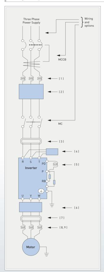
The sensitivity of circuit breaker (MCCB) should be differentiated by the sums of wiring distances (inverter-power supply and inverter-motor).
