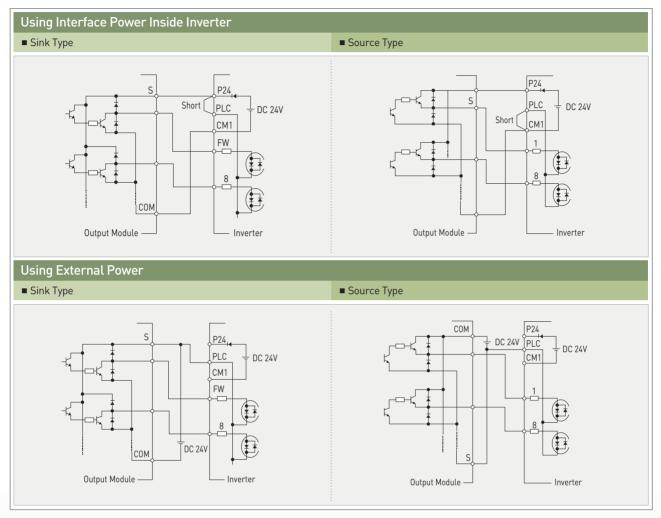
\*\* Be sure to turn on the inverters after turning on the PLC and its external power source to prevent the parameters in the inverter from being modified.
